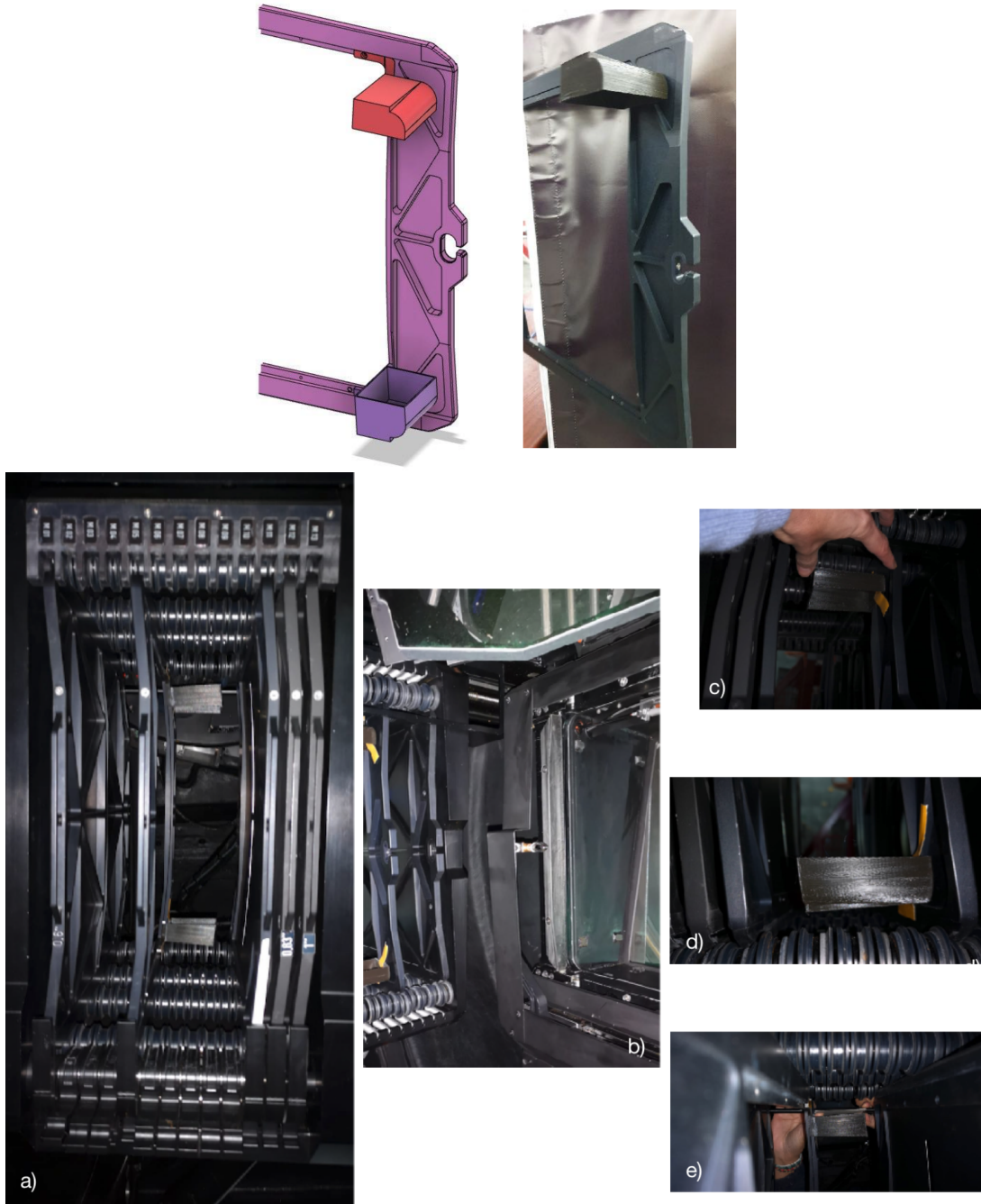
Figure 25. Top: 3D printed dummies built for the in situ testing of the MAAT envelope on OSIRIS (Credit: GTC). Bottom: In situ testing of the dummy of the MAAT module on OSIRIS: a) MAAT envelope dummy placed in the Loader mask, b) Baffle to redesign in order to accommodate the subsystem mask frame plus MAAT envelope, c) Width of the MAAT envelope, d) Free space between the rollers and the lower part of the MAAT envelope (orientation rotB = 80^\circ ), and e) Free space between the upper part of the MAAT envelope and the masks edge protection (orientation rotB = 80^\circ ). All these pictures have been taken with orientation of rotB = 80^\circ . (Credit: GTC).
