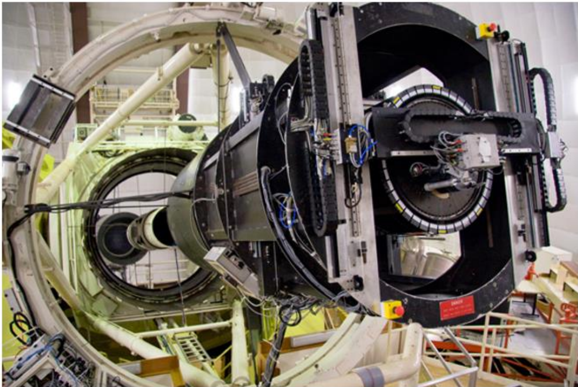
Figure 41. The 2df fibre positioning system at the Anglo-Australian Telescope.
